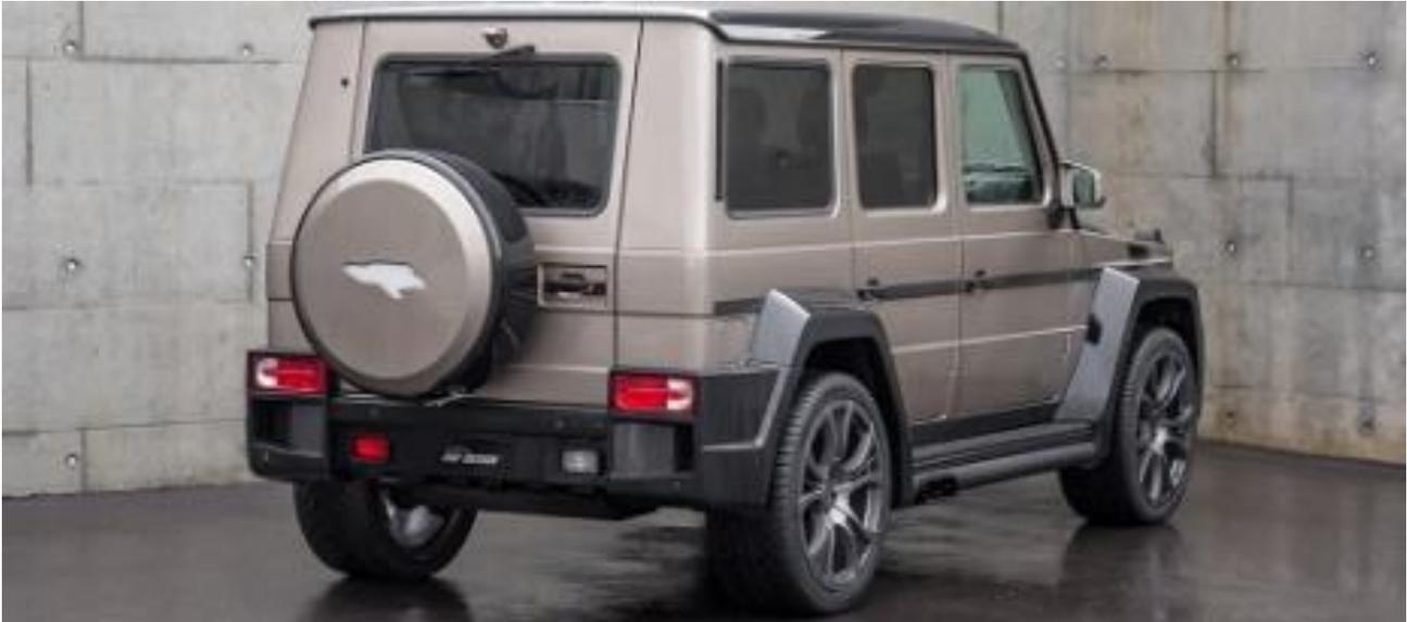
The new 11x23 inch FAB Design "EVOTREK" wheel, made in forged monoblock technology for tyre size 305/35R23, recommending ADVAN S.T. tyre from our technology partner Yokohama. The high-grade manufactured wheels show a low wall-thickness, they are 40% lighter than the traditional casted wheels and they reach extremely high load index. Thereby those FAB forged wheels are qualified for all Mercedes, Land Rover- and Porsche SUV-models.
