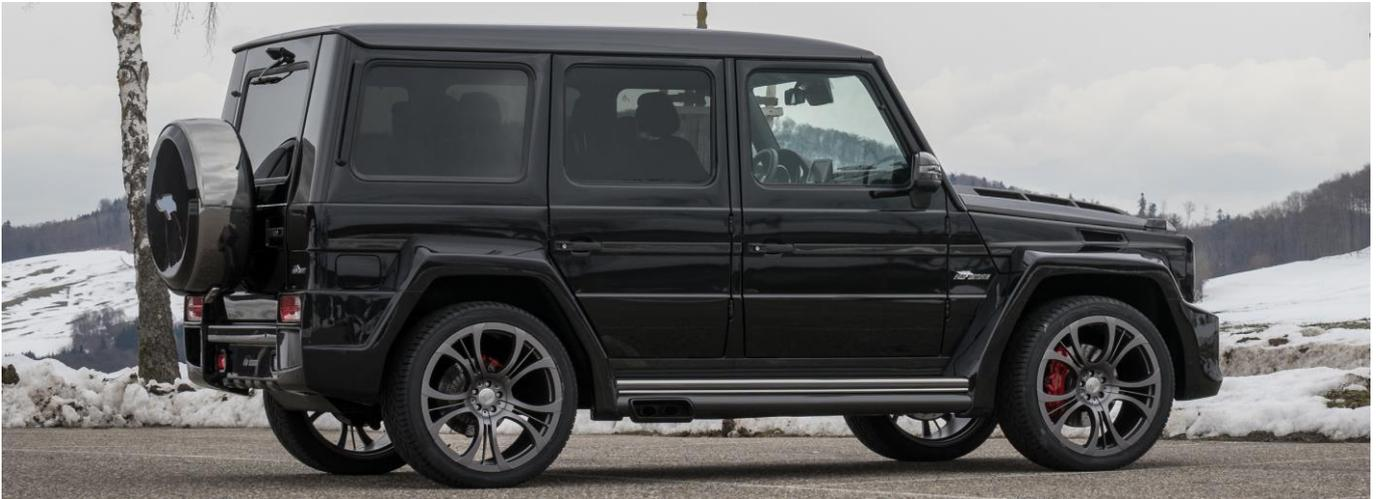
The large and wider wheel arches are filled with forged monoblock wheels in sizes of 11 x 23 inches, which are covered with 305/55 R 23 size tyres. The time-consuming production process guarantees the excellent qualities of the high-performance rims. During the forging process, the material is compressed to a point where all air inclusions are forced out of the aluminium.
